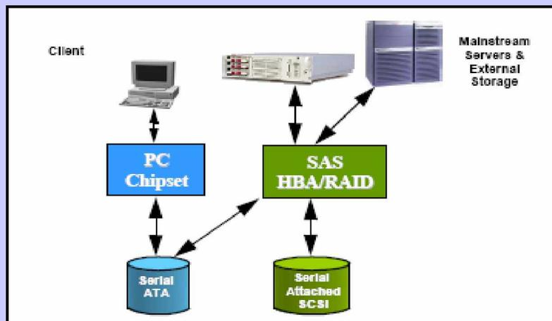
Figure 1. Serial ATA/Serial Attached SCSI Compatibility
