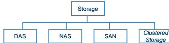
Clustered storage architectures have the ability to pull together two or more storage devices to behave as a single entity. Clustered storage can be broken down into three types:
