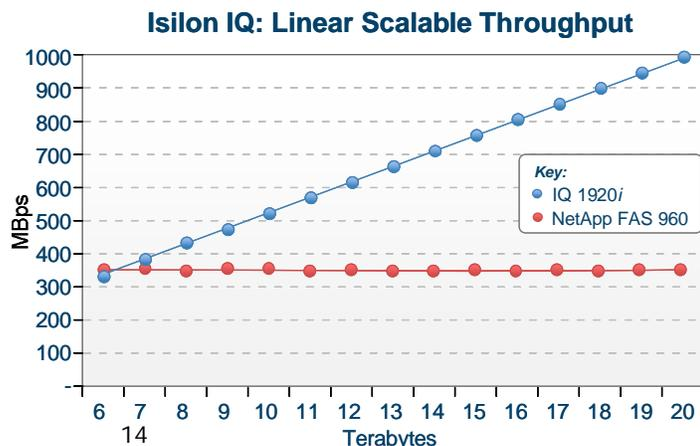
memory, CPU power, journal space and disk spindles. A new Isilon IQ node equips the aggregate of the cluster with approximately 700 megabits per second of available throughput that scales linearly, allowing customers to easily meet increasing bandwidth needs.
